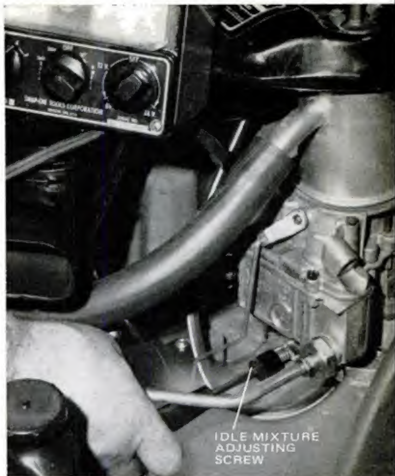
CARBURETOR ADJUSTMENT is made using tachometer to get right idle mixture for optimum performance
